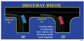
Adequate driveway width can help turning vehicles get off the road with a greater speed and less encroachment into oncoming driveway traffic.
