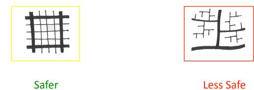
Within each type of street pattern increasing connectivity – measured by link-to-node ratio - was not correlated with improved safety
