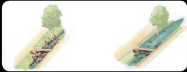
VEGETATIVE STONE SWALE - DRY AND WET
