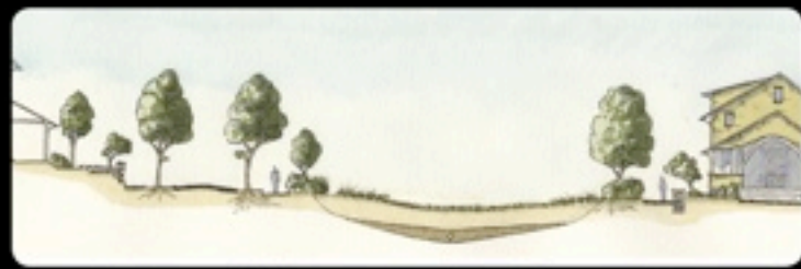
T3 - BIO-RETENTION SWALE - DETAIL
